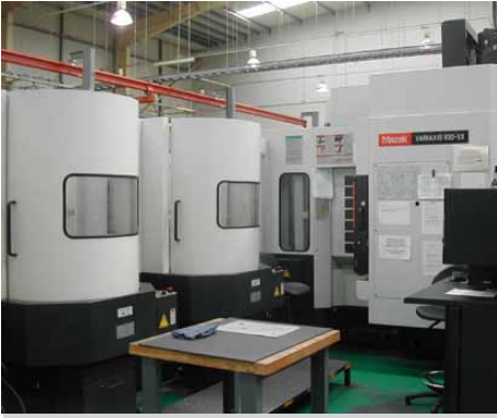
Bromford's flexible manufacturing system (FMS) is built around a 5-axis MAZAK Variaxis 630 machining center
